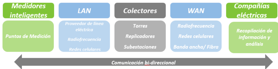
Figure 8: AMI communication layers, Carbon Trust analysis
