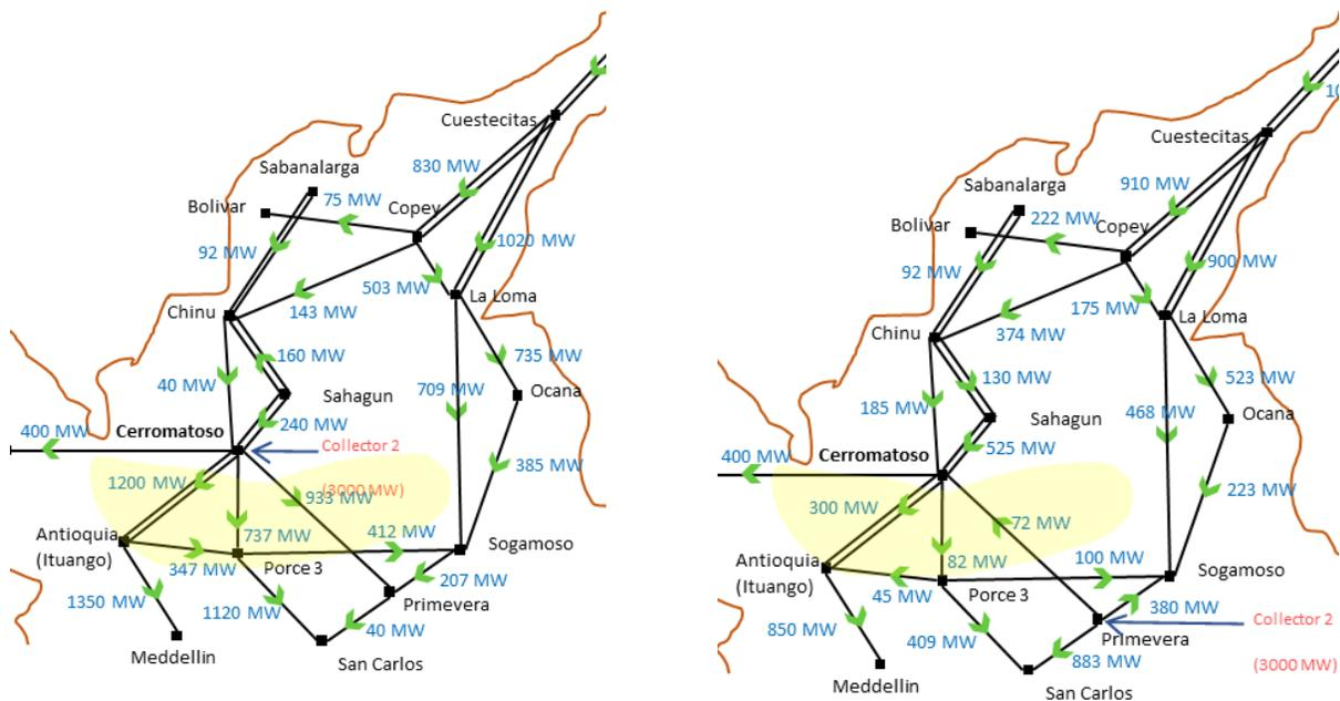
**Figure 4-3 Power flow comparison-Collector 2 interconnected at Cerromatoso vs Primavera (2032 Max Dem Max Gen)**
