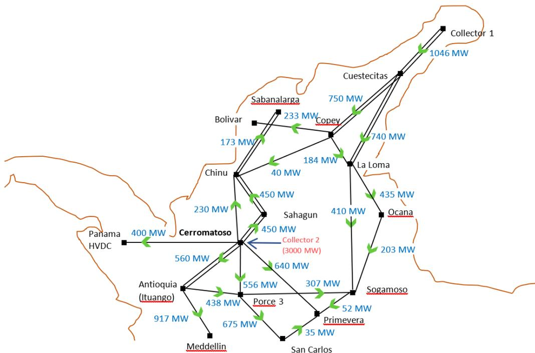
Figure 3-3 Active power flow on selected 500 kV transmission corridors - 2032 Min Dem Min Gen
