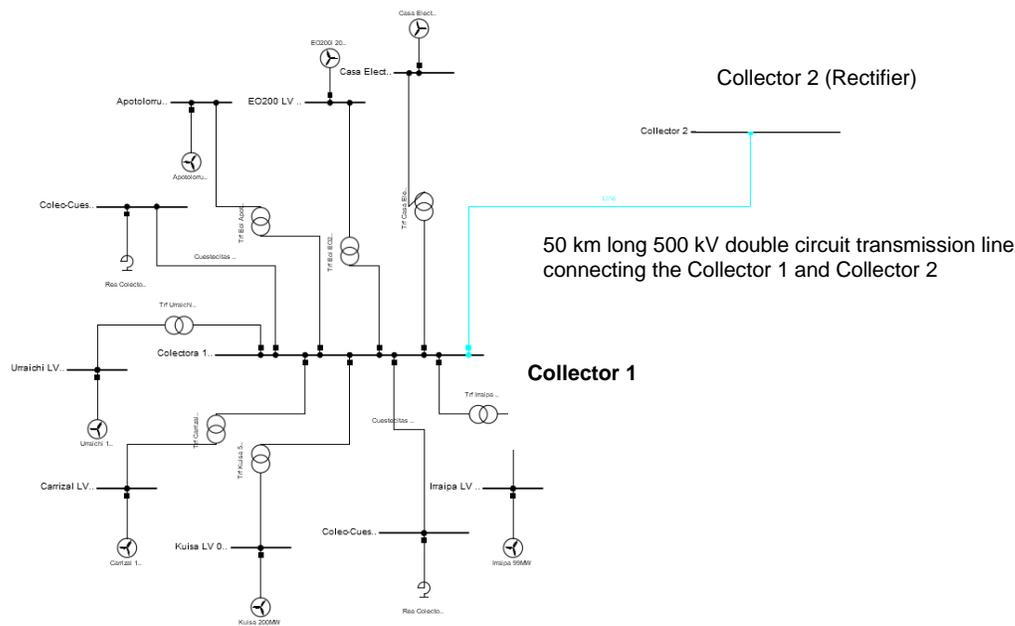
Figure 3-12 LCC HVDC transmission system rectifier at the Collector 2
