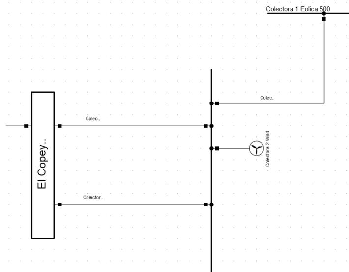
**Figure 3-8 Collector 2 interconnection to Copey using 500 kV double circuit AC transmission lines**
