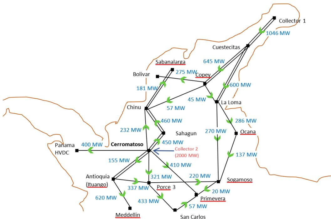
**Figure 3-1 Active power flow on selected 500 kV transmission corridors - 2028 Min Dem Min Gen**
