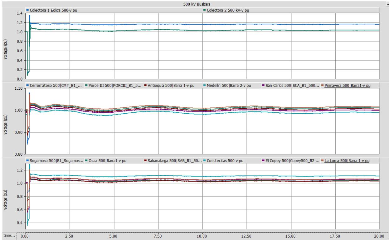
Figure 3-10 Selected 500 kV bus voltages (Contingency 1, 2032 Max Dem Max Gen—Alternative 4)
