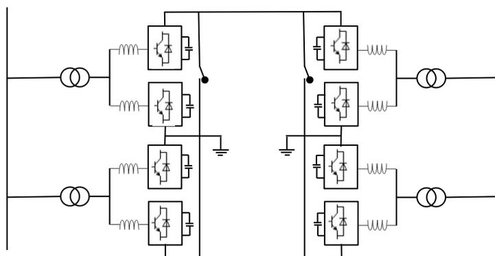
**Figure 4-4 Simplified diagram of a VSC HVDC bipole system**
