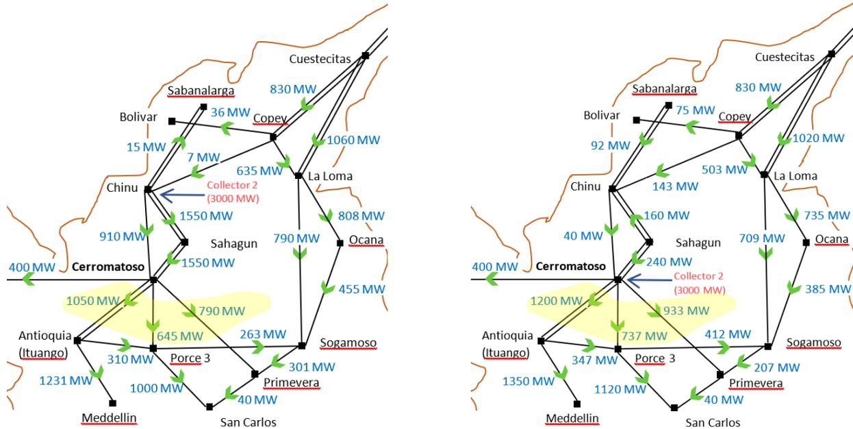
**Figure 4-2 Network power flow based on the Collector 2 interconnection location in 2032 Max Dem Max Gen study case (Left: at Chinu, Right: at Cerromatoso)**
