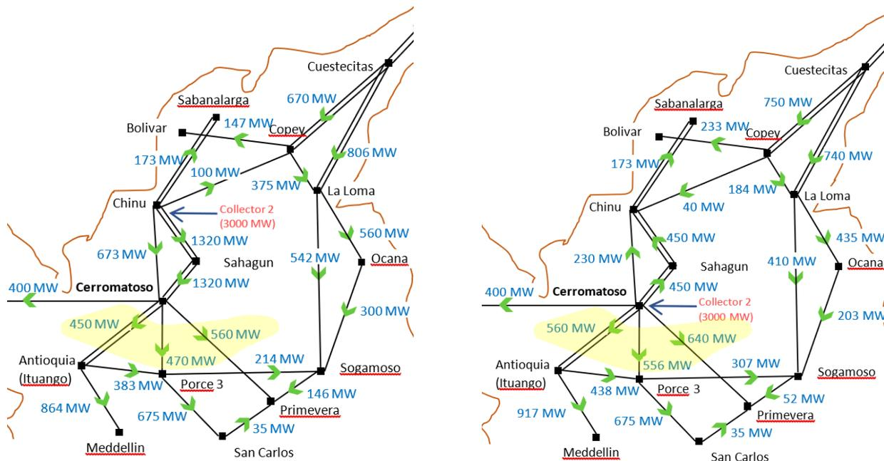
**Figure 4-1 Network power flow based on the Collector 2 interconnection location in 2032 Min Dem Min Gen study case (Left: at Chinu, right: at Cerromatoso)**
