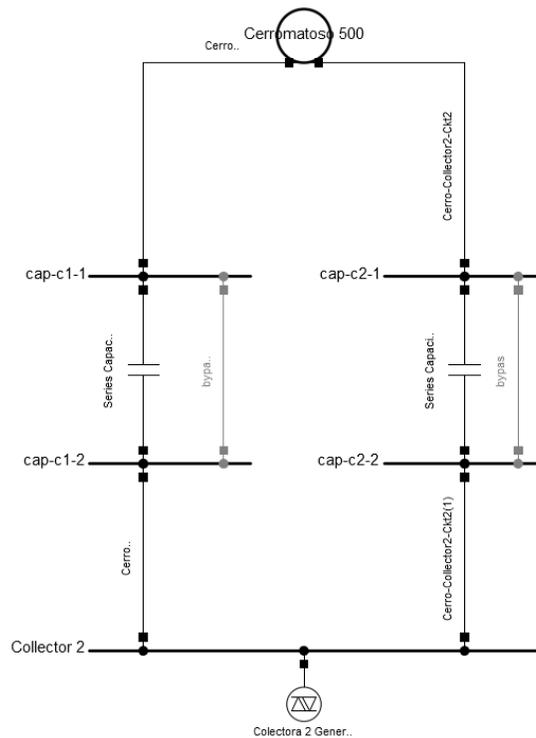
**Figure 3-7 650 km long 50% compensated 500 kV double circuit transmission line from Collector 2 to Cerromatoso**
