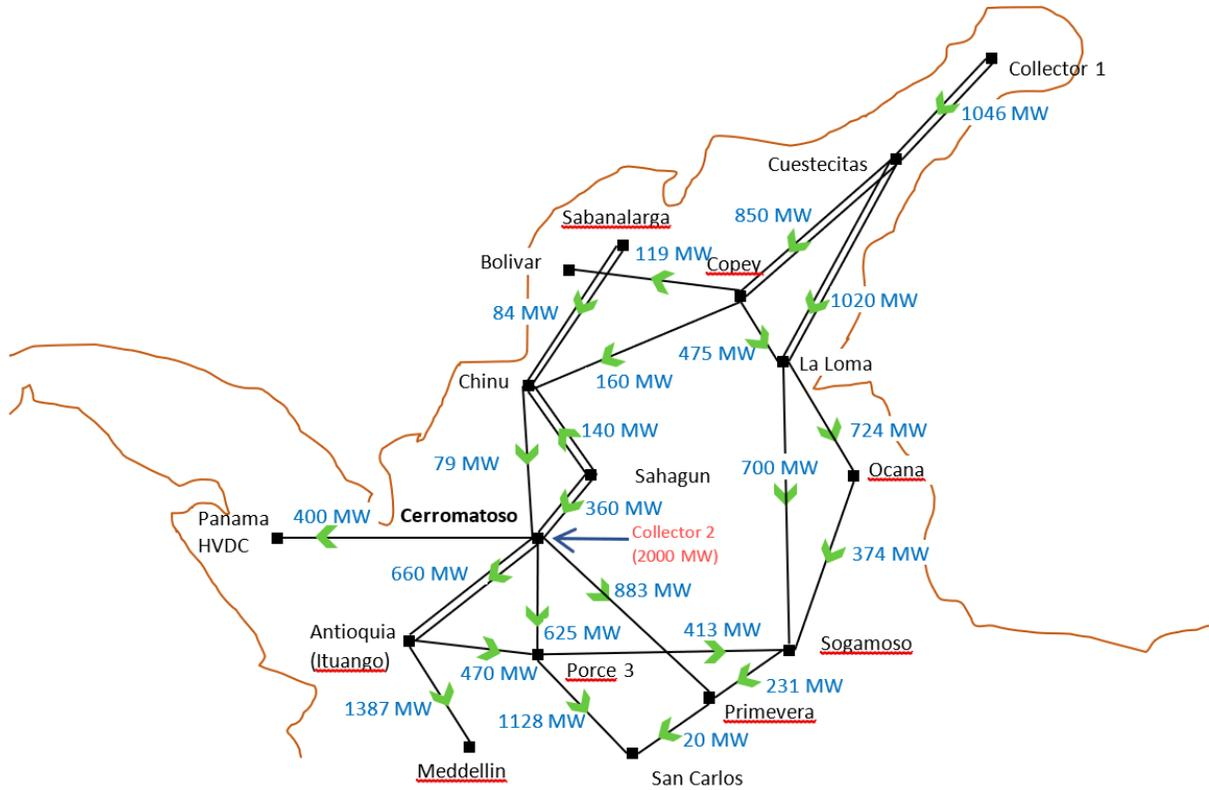
Figure 3-2 Active power flow on selected 500 kV transmission corridors - 2028 Max Dem Max Gen
