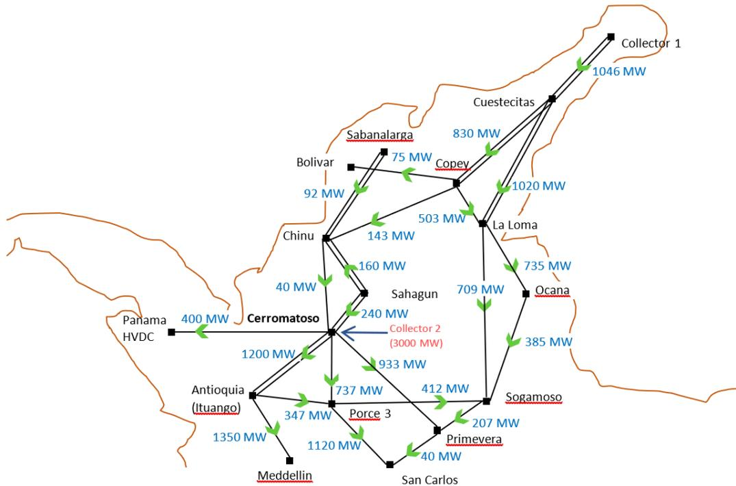
**Figure 3-4 Active power flow on selected 500 kV transmission corridors – 2032 Max Dim Max Gen**
