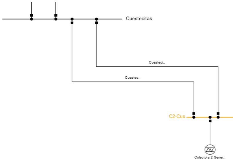
**Figure 3-6 170 km long 500 kV double circuit transmission line from Collector 2 to Cuestecitas**
