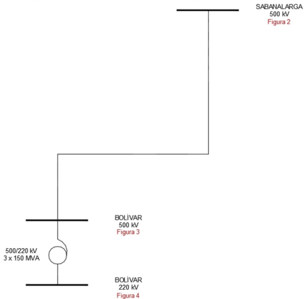
FIGURA 1. DIAGRAMA ESQUEMÁTICO
